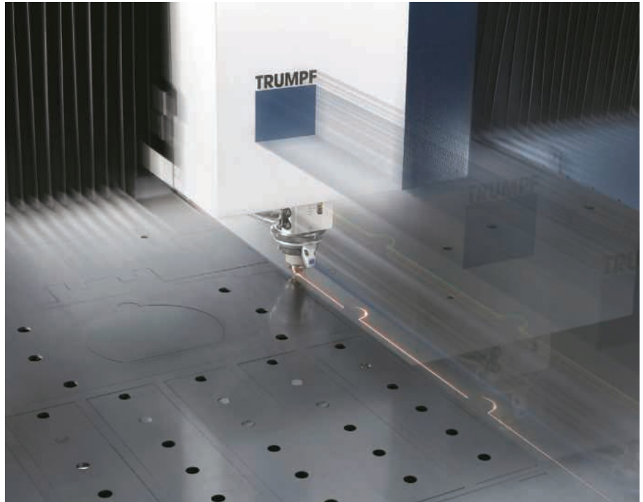
The Highspeed cutting process can nearly double sheet throughput compared to standard cutting. A bi-flow nozzle reduces gas consumption by 40 percent on average
