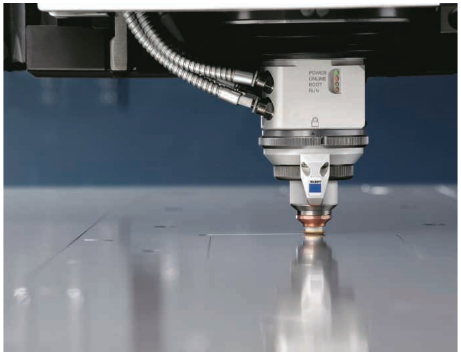
A newly designed nozzle reduces nitrogen consumption by 70 percent on average in the Highspeed Eco process. As with the Highspeed process, feed rates and sheet throughput increase by as much as 100 percent
