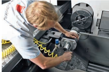
An integrated rotary axis on the Bystronic ByStar Fiber and a setup assistant facilitate rapid transition between sheet and tube cutting
