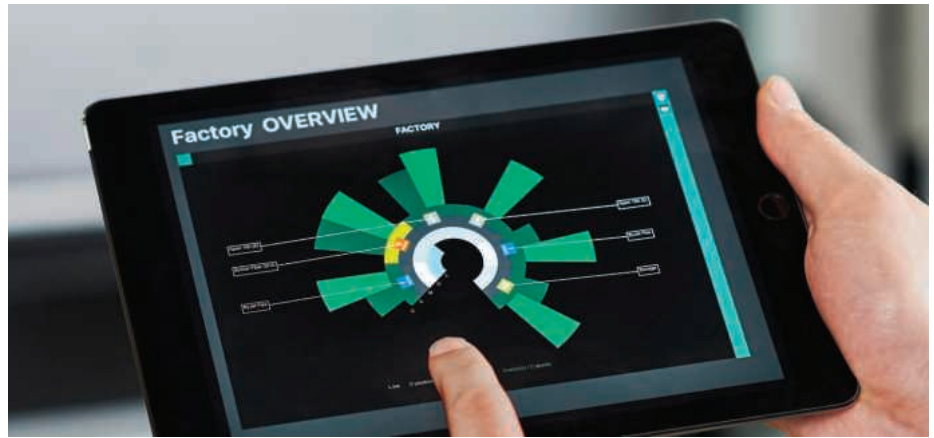
The sunburst view is one of several status reports in Bystronic's ByCockpit software. It displays the condition of an entire factory at a glance
