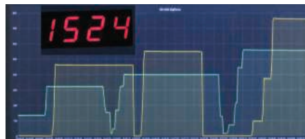
On-screen digital readout of clamping force from two Digiforce devices
