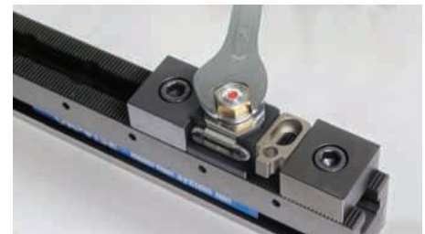
The OK-VISE Dotforce allows the holding pressure to be verified of workpieces that have been manually secured in a Multi-Rail RM workholding system
