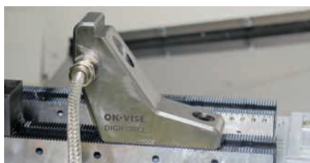
A Digiforce device for measuring how securely a component is clamped in an OK-VISE Multi-Rail RM workholding system
