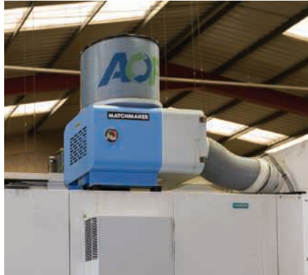
The oil mist filtration systems supplied by Matchmaker CNC are improving the environment and productivity at Nasmyth Arden
