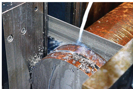
Thanks to the powerful coolant pump and large coolant tank, the saw blade is protected even when cutting difficult-to-machine materials
