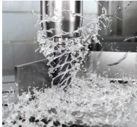
The new CoroMill® Plura HFS ISO S cutters from Sandvik Coromant are ideal for machining aerospace components made from titanium- and nickel-based alloys
