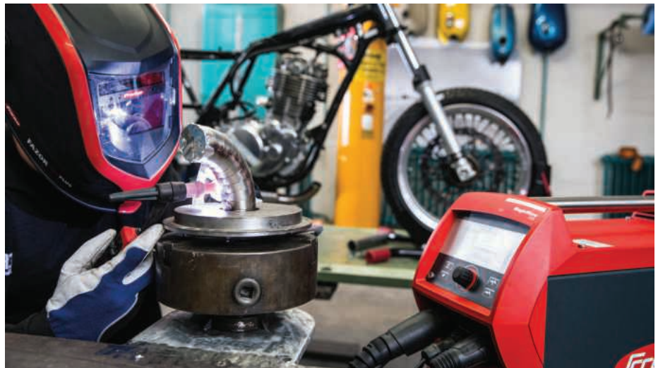
The MagicWave 230i can communicate with other devices via Bluetooth, WLAN and NFC technology, and can be networked with them
