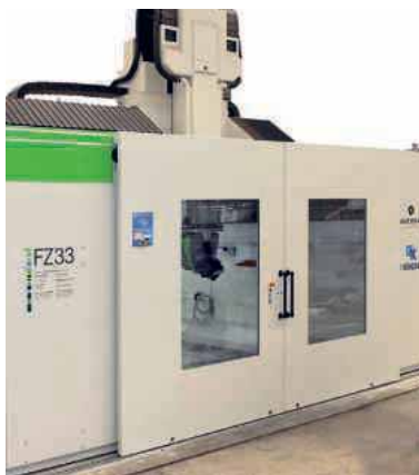
One of the Zimmermann FZ33 portal, 5-axis machining centres for producing large composite aircraft components
