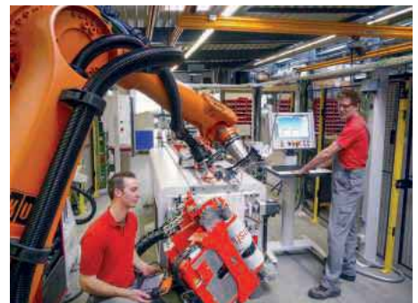
As with any conventional bending machine, the necessary data may be loaded into the bending robots with a data file directly from the CAD system and transformed into a bending geometry
