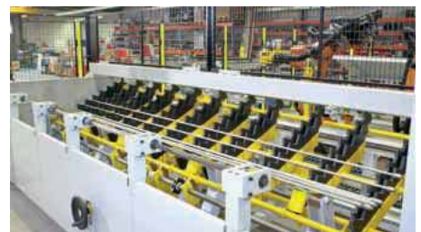
One magazine is a so-called step conveyor. It guides pipes to the bending robot
