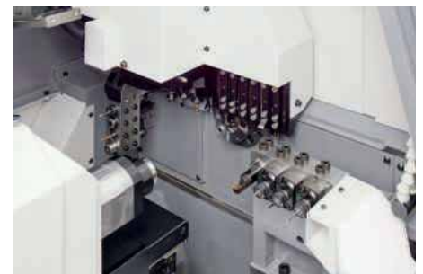
Citizen's Cincom D25 has 10-axes controlling two gang vertical toolposts plus back toolpost and opposite toolpost
