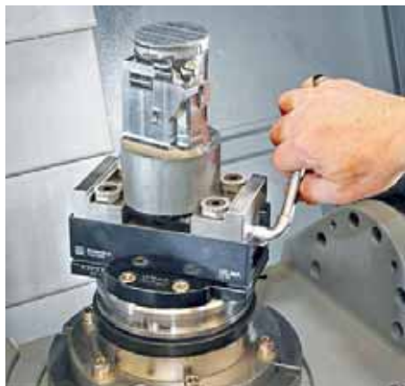
The Roemheld PC80Z self-centring vice in its new configuration with round inserts clamping a cylindrical component
