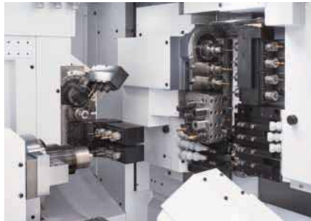
The Citizen Cincom L12-VIII LFV can accommodate up to 27 tools and can be specified with 16 mm bar capacity
