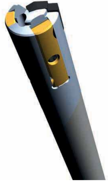
WP-ELB series 10 drilling tool: The TBT indexable insert single-lip drills also include replaceable carbide guide rails to guide the tools in the bore. The strips additionally smooth the bore, which is why the best surfaces are created
