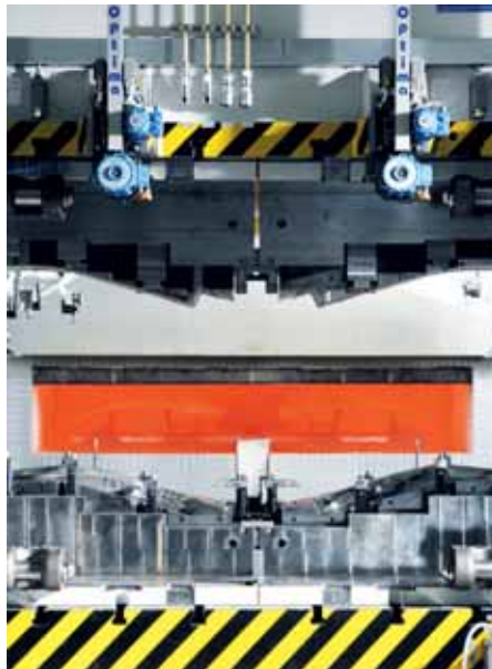
Press hardening tool made of Thermodur 2383 Supercool
