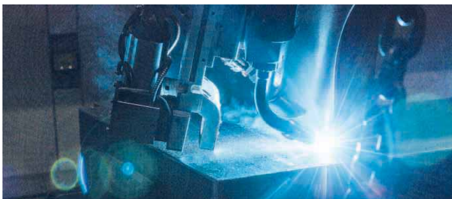
The laser beam heats the surface of the component, resulting in deep, narrow penetration. The arc then forms a wide weld pool to provide outstanding gap-bridging ability
