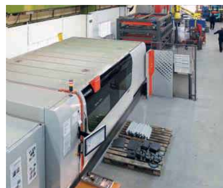
A view of the ByStar Fiber at Stevens & Carlotti, Sandwich, showing the ByTrans Extended auto sheet load / unload equipment in the background
