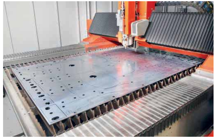
A 6 mm mild steel sheet being processed in the ByStar Fiber
