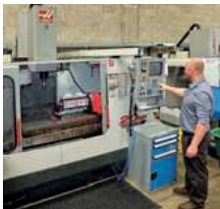
Jonathan Caple operating the Haas vertical machining centre on which the tombstone and trunnion arrangement from 1st MTA has been fitted
