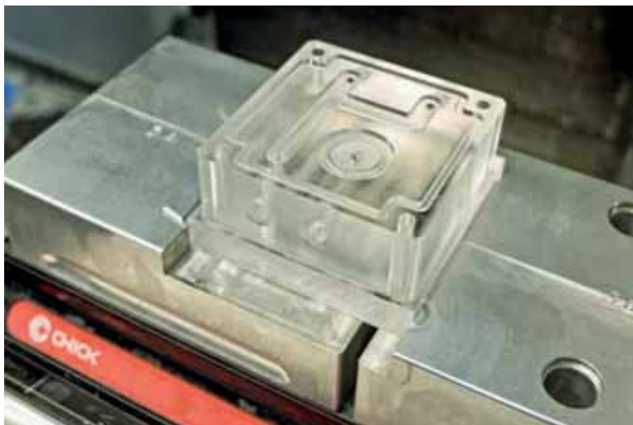
One of the acrylic manifold blocks machined in one hit on three sides. The component sits high in the machined soft jaws, allowing tools access to the top, front and back
