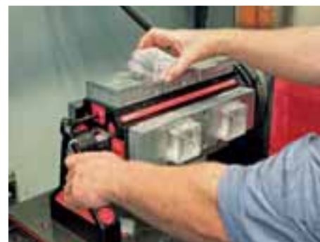
Machined manifold blocks being unloaded ready for material to be milled from the back in a second operation
