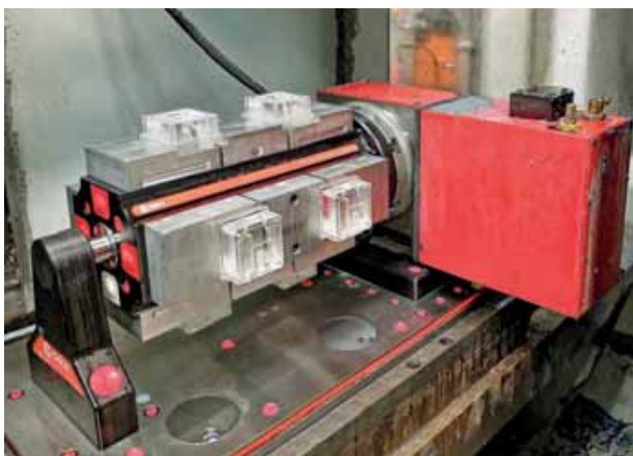
Close-up of the Chick Indexer Subsystem, with a Multi-Lok holding two acrylic manifold blocks on each of four faces in Qwik-Lok clamps
