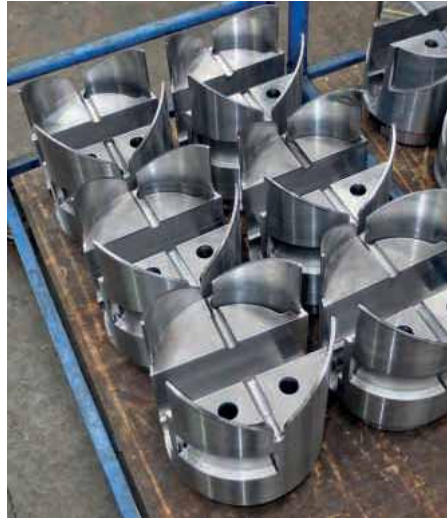
Another example of the use of NC Merge in WinMAX. The component is an oil and gas industry part machined from a solid billet of AISI 4140 steel
