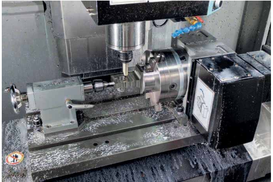
A close-up of the Hurco 4th axis rotary table and tailstock securing a 316 stainless steel wheel bracket, part of a remotely operated vehicle for the offshore industry
