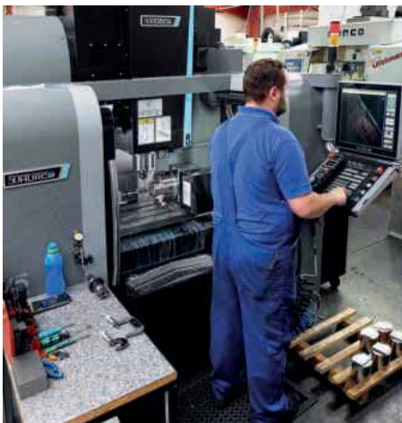
One of a pair of Hurco VM10i vertical machining centres, equipped with a 4th CNC axis, purchased by Cowie Engineering in 2018
