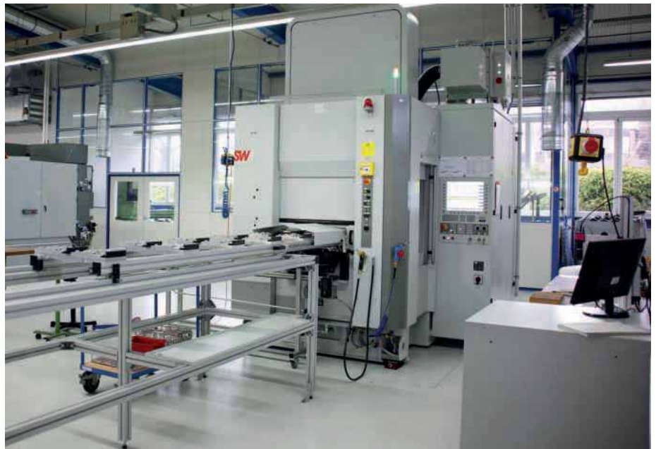
The fully automated SW BA 321 dual-spindle machining centre produces two completely machined forceps halves every three minutes. Source: Klaus Vollrath
