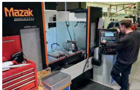
The Mazak VCN-530C 3-axis VMC in use at Axminster Tools & Machinery
