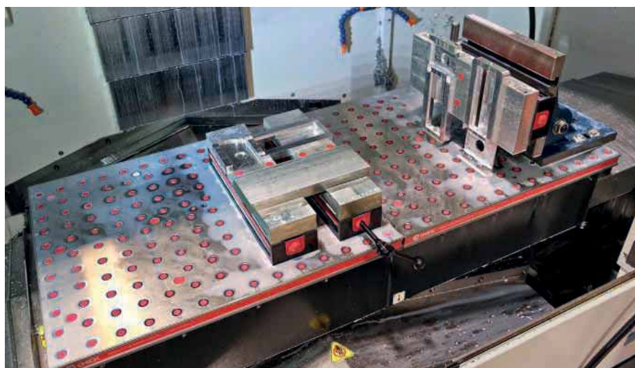
The two-part CHICK foundation plate fitted to the VCN-530C contains an array of holes 11 deep by 27 across. Here a grooving jig for a router is being produced in three operations by clamping the aluminium component in three CHICK Qwik-Loks
