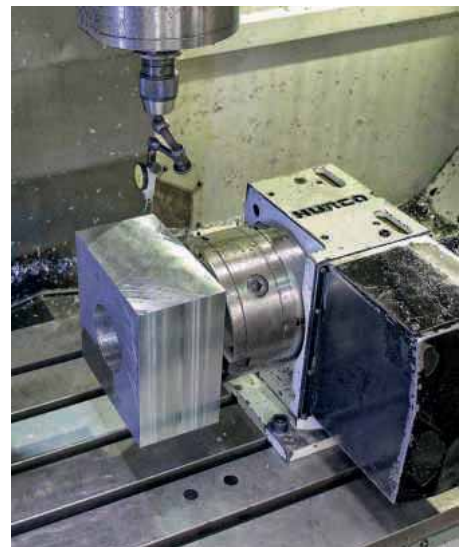
Close-up of the manifold casing secured in the Hurco 4th axis
