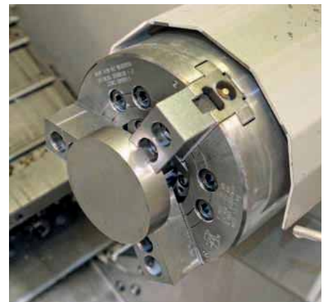
Also supplied by 1st MTA to Axminster Tools & Machinery are machinable steel jaws for the chucks in the manufacturer's twin-spindle Mazak turning centres. Here a stainless-steel billet is ready for Op1 machining in the sub-spindle
