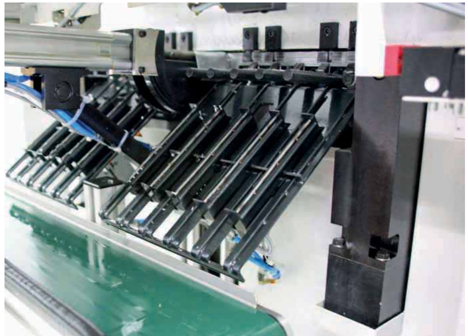
An elaborate drawer mechanism ensures controlled deposit on a conveyor belt. Source: Klaus Vollrath
