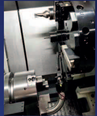
The 12 Station Turret and the Automatic Tool Pre-Setting Arm gives the operator consistency when measuring tool offsets.
