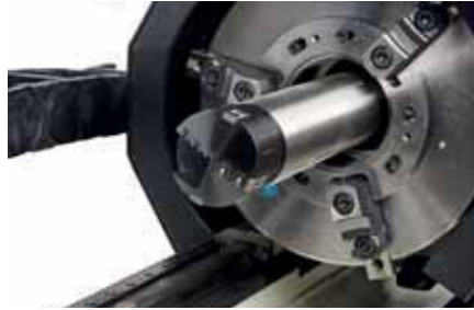
Standard heavy-duty 3-jaw chuck
