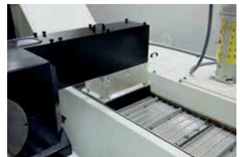
Automatic chip removal system
