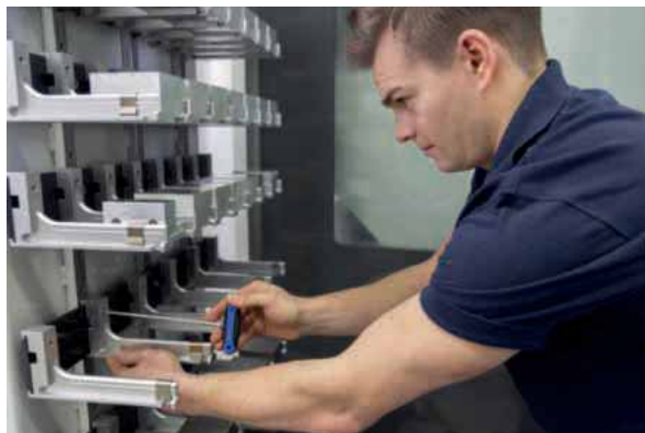
Material rack layout easily changed to accommodate varying workpieces
