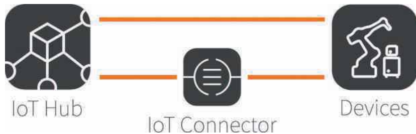
The devices can be connected either directly to the IoT Hub or to an additional IoT Connector
