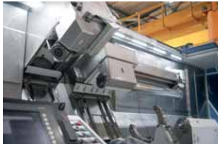
The main components such as the boring bar slide and the turning-boring-milling unit have been completely renewed
