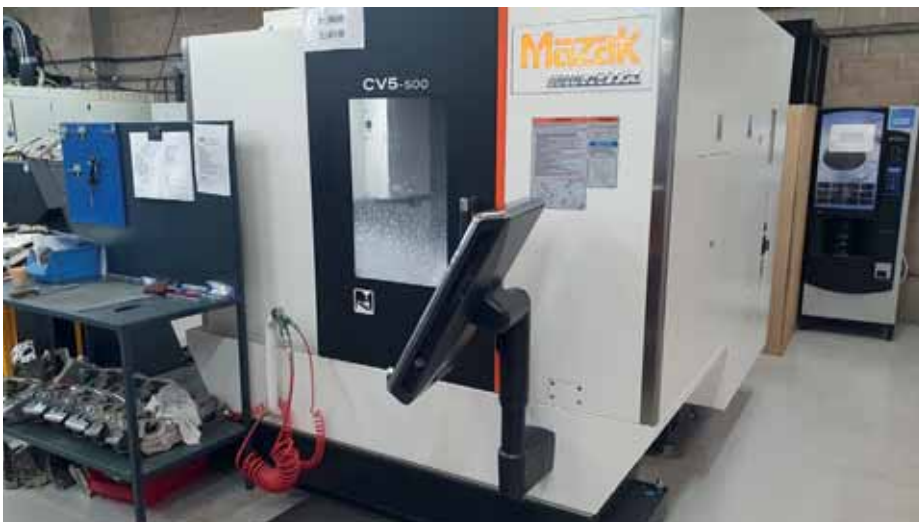
With convenience and additional machining capability in mind, NuMachine opted to invest in two CV5-500 units - Yamazaki Mazak's newest fully simultaneous 5-axis machining centre
