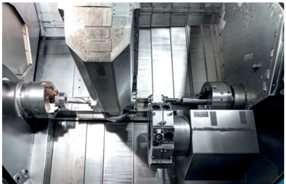
Up to nine machining axes including the option of 5-axis interpolation was possible at WFL even 25 years ago. The design with the bottom tool turret and counter spindle allowed for maximum productivity and flexibility
