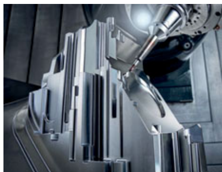
The headlamp lens mould machined with various different types of Horn end mill
