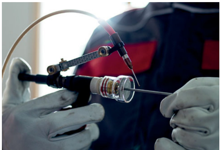
The patented TFC electrode clamping system releases and clamps the tungsten electrode at the touch of a button, allowing it to be changed in a matter of seconds
