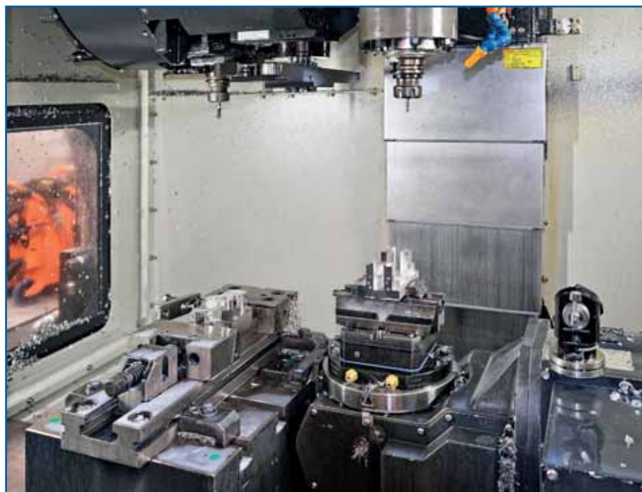
The V-30iT is unusual in that the left-hand side of the swivelling trunnion with rotary table is supported by a bearing in the side of an adjacent fixed table, so 3-axis machining and 3- to 5-axis machining on the same part can be completed without it leaving the working area. Alternatively separate jobs may be undertaken on each table
