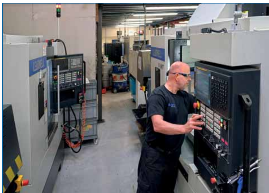
The pair of Leadwell V-30iT 5-axis machining centres on the shop floor at G&J (CNC) Services' Paddock Wood factory. The compact machines, each of which occupies a footprint of just over 2.4 by 2.1 metres, raised the number of CNC machine tools on site to 18
