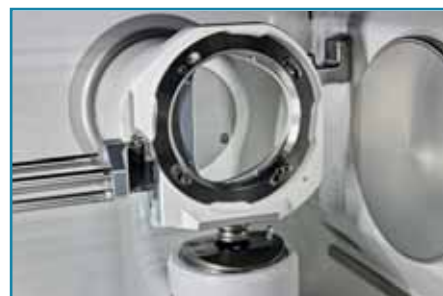
A material holder in the Ceramill Matik being located accurately in the Stark zero-point clamping system. Prior to prosthesis production, a material blank is inserted into the holder
