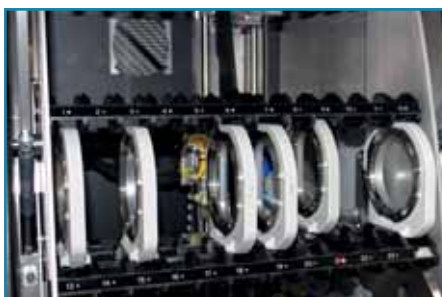
Up to 36 workpieces may be held in the material magazine, allowing extended periods of unattended machining
