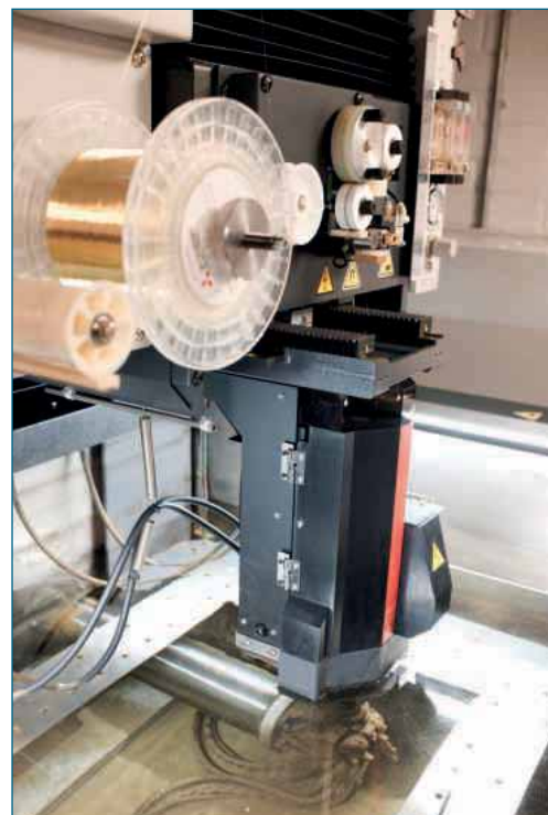
The Wire Feeding System on the Mitsubishi Machine
