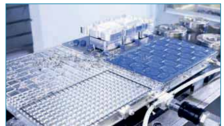
The SFM FlexMat, shown in blue here, can be used as an alternative to the ISBL vacuum blocks
