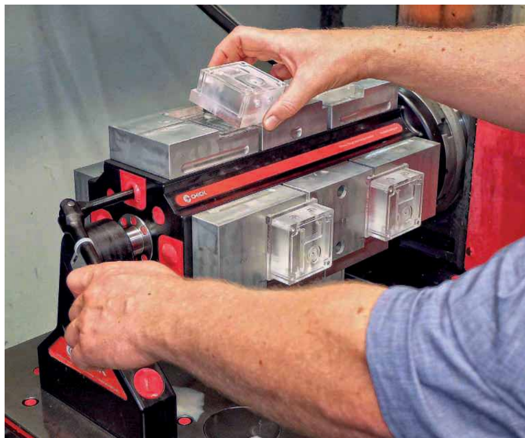
Machined acrylic manifold blocks being unloaded from the Chick ISS at subcontractor Stratos Precision Engineering, Gloucester. The components sit high in the machined soft jaws, allowing tools to access the top, front and back. A 4-sided ISS like this is the norm, although 6- and 8-sided versions are also available
