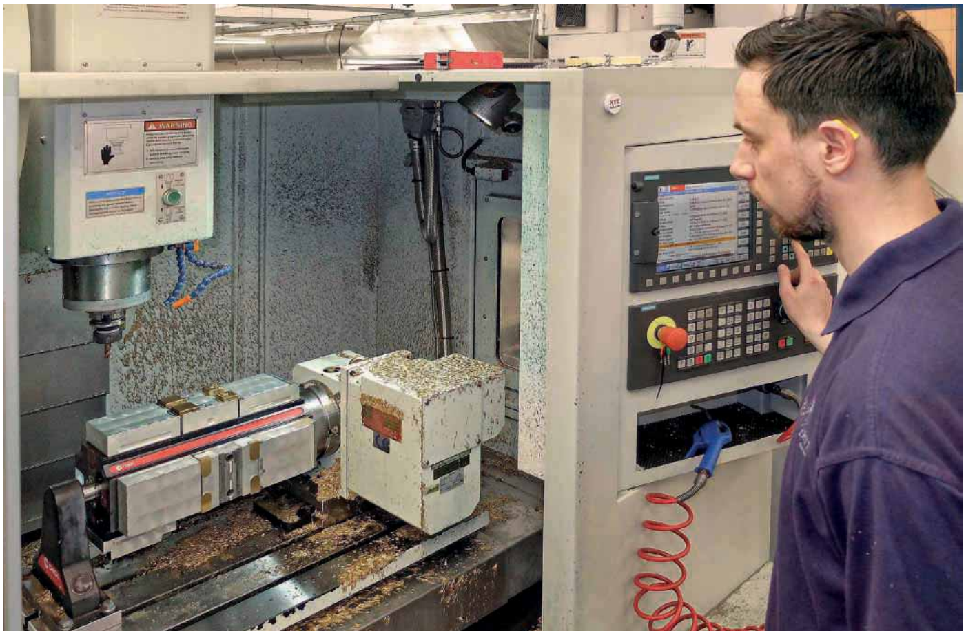
Dissimilar brass fittings set up for machining on a Chick ISS on one of the VMCs at Armac Martin, Birmingham. After the faces of the first set of parts have been machined, one or two edges of each component can be accessed after indexing, reducing the need for additional setups
