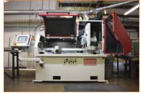
The VA-L 560NC is a circular cold saw specifically geared toward aluminum and is suited for Kyser's specific production needs
