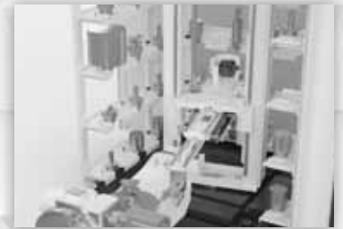
32 position Auto Work Changer (AWC) (max. workpiece Ø350 x H315 x 65kg)
