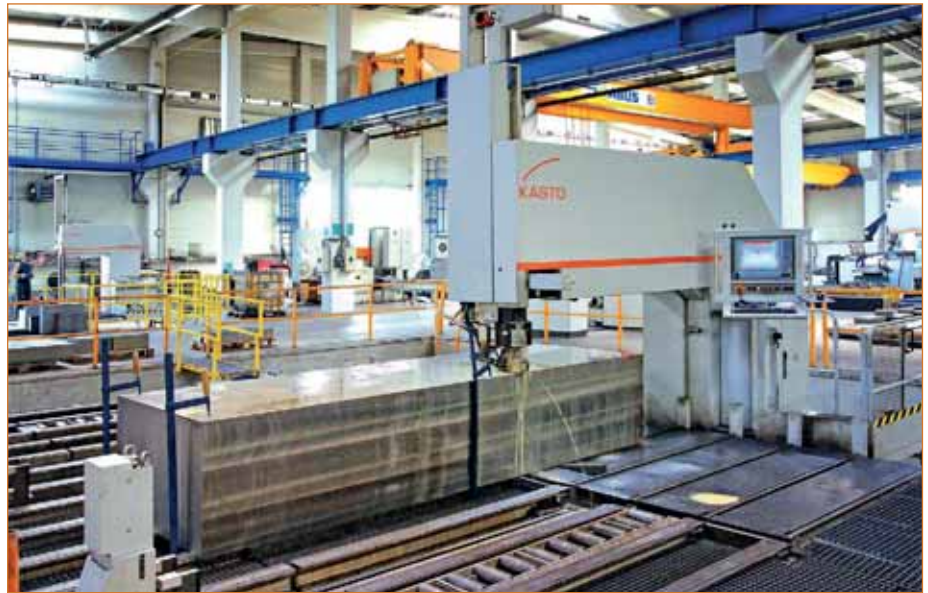
Steel stockholder JKZ Bučovice uses KASTOObbs block bandsaws to cut large, heavy workpieces
