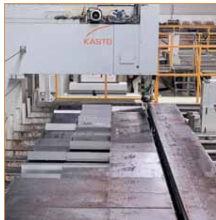
The KASTOObbs is designed to process billets or plates of various geometries, grades and dimensions
