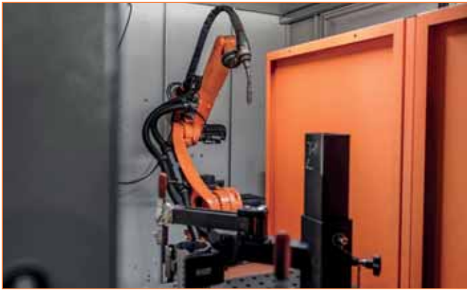
The robot improved sheet metal working processes significantly through automated welding
