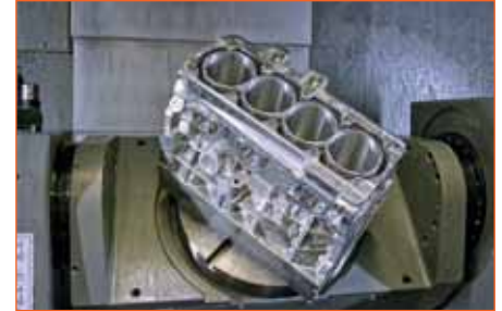
An aluminium block for an A&M EDM Ascaso A+5 1273 cc K16V turbo engine on the table of a 5-axis Hurco VMX42Ui VMC
