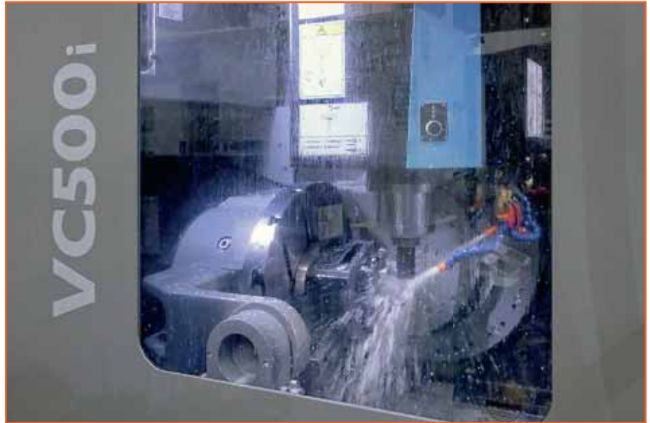
The Hurco VC500i 5-axis machining centre in operation at Wellington Engineering, Hayes
