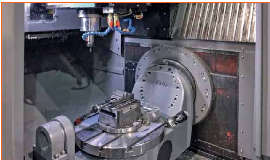
Working area of the 5-axis VC500i, showing the rotary table / swivelling trunnion positioned from front-to-back, instead of in the more usual side-to-side arrangement. Doors on two sides open to allow ergonomic operator access
