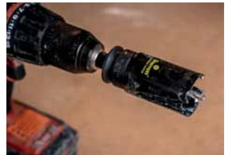
The MPH saw has a depth of 54 mm, 2.1/8"
