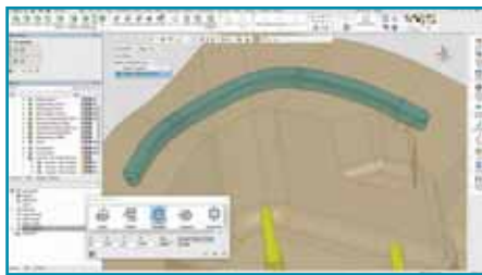
Construction of 3D runner design based upon constant volume of vertical orientation and section orientation
