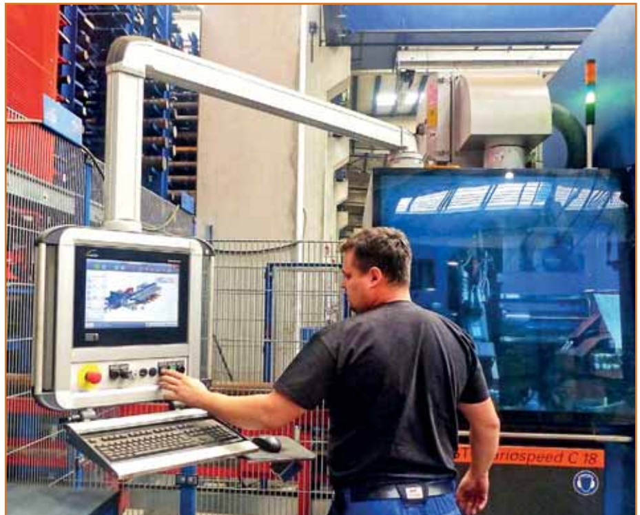
The new KASTOvariospeed C 18 automatic circular sawing centre at Bieber + Marburg
