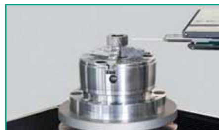
Measurement in machining direction in the smallest tooth flanks, module 1 and higher
