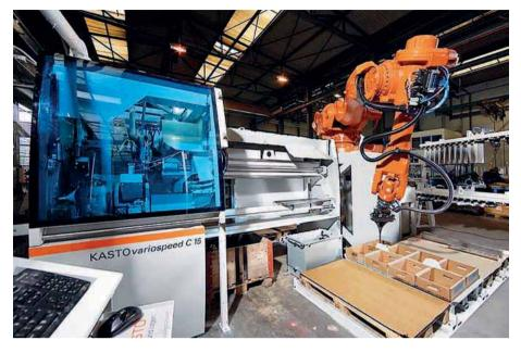
sawing machine can run attended, with the control system holding all parameters of a job including material diameter, band speed, rate of downfeed, cut length and number of parts.
