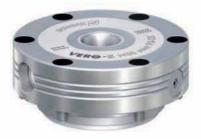
VERO-S NSE3 is a new flagship for quick-change pallet technology. SCHUNK has yet again boosted the performance characteristics of the VERO-S NSE3 138 as compared against previous top sellers. An enormous pull-down force of 8,000 N or 28,000 N with activated turbo function as well as increased dimensional stability for the module body have a positive impact on the rigidity of the clamping solutions.
