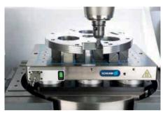
demanding applications. Due to the conical fitting, the clamping pins can also be joined into the modules eccentrically, making this process incredibly easy. The actual clamping is done via spring force without any external energy supply; it is form-fit and self-locking. The workpieces remain safely clamped in case of a sudden pressure drop in the air system. A pneumatic system pressure of six bar is sufficient to open the clamping modules.
