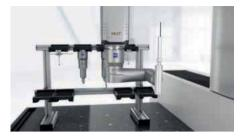
advantages to customers. Unlike with a CFS sensor, operators using the ZEISS DotScan can switch it in and out as needed.
