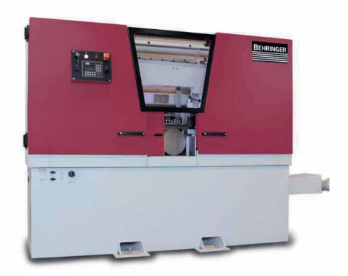
of vibration-damping grey cast iron and double band wheel bearings work together to ensure quiet running and cutting precision. Trials confirmed a 30 percent longer service life of bandsaw blades alongside visibly better cut surface quality. The slight inclination of the band wheels helps prolong the life of bandsaw blades by reducing fatigue due to cyclical bending.
