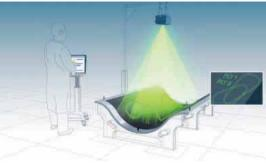
For large assemblies and/or in space-constrained areas, multiple TracerM projectors can be controlled from a single workstation to provide large-scale virtual templates in one coordinate system.
