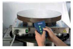
To ensure process reliability in automated applications, it is possible to monitor each individual magnetic chuck. To do this, the individual clamping state is transmitted via a PLC interface to the system control. The SCHUNK MAGNOS KEH plus control unit is completed by the handheld remote SCHUNK MAGNOS HABE-S plus that is also modular. This allows control of the individual magnetic chucks and the individual 16-step holding force regulation process.
