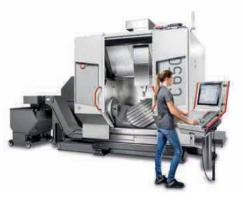
Standard CNC system is Heidenhain's TNC 640, which offers the full programming capability of this proven, high-end control. The GUI has a large, full colour, 19" TFT flat panel monitor and the control can be swivelled to the magazine loading station so that the operator can enter tool data directly into the control.
