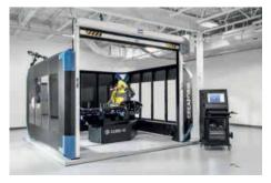
software calculates the most efficient positioning of the sensor and the best collision-free trajectories for the robot; the same software manages the optical 3D measurements, simultaneously provides advanced analysis of the results, even when computing huge point clouds; it edits personalised, easy-to-understand reports. In short, the Metrolog and Silma X4 i-Robots turn the CUBE-R into a simple automated measurement solution, easily operated by a non-specialist operator.
