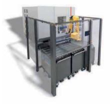
An intuitive, easy-to-operate touch panel enables easy control of the automated system and, as external access to the trolley is possible, production remains seamless as machining cycles do not need to be interrupted. Control of the zero-point clamping system can be performed either pneumatically through the machine tool or mechanically through the system's robot.
