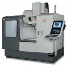
range is the XYZ 660 HD, which features increased X and Y travels over its predecessor of 660 mm and 450 mm, yet retains a compact footprint making it ideal for most machine shops, while the XYZ 1100 HD replaces the earlier 1020 machine and now has X and Y travels of 1,100 and 610 mm respectively. The full range is the XYZ 660 HD, 800 HD, 1100 HD, 1510 HD, along with three 'super-heavyweight' machines, the XYZ 2010, 2510 and 3010 HD completing the line-up.
