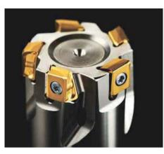
A single flat rake face on the insert improves chip disposal and provides accurate wall face step overs with a cusp height of only 8  $\mu$ m when deep wall machining. Additionally, the minor cutting edge that blends smoothly into a large corner radius also provides a benefit by providing the ability to achieve good component surface finishes. The top face geometry combines the minor cutting edge and a relief angle that makes ramping possible.
