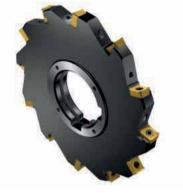
Ease-of-use is a further requirement of machine shops the world over. For this reason, CoroMill 331 makes use of spring-loaded cassettes with serrations that provide security and easy setting for the desired width. Moreover, a pin-controlled adjustment range enables manufacturers to set the cutter with high accuracy for precise groove dimensions.
