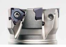
geometry, but also generate low cutting forces, ensuring smooth machining coupled with high levels of productivity. This is an important user benefit, particularly in cases where less powerful machines and unstable workholding are being used.
