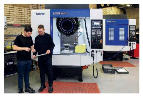
Since the machine was installed, CTPE has gone a step further by optimising the program to machine six parts on the table with 14 tools and adopting new types of cutters. The effect has been to reduce the cycle time per part further to just 30 percent of the original.
