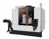
Also on display was the VCN-530C, a UK-built vertical machining centre powered by a high-speed 18,000 rpm milling spindle
