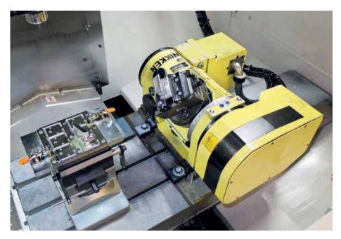
produced in three operations on a 3-axis machine in 15 minutes and is now produced in an Op1/Op2 cycle on an S700X1 in six minutes, representing a 60 percent time reduction.
