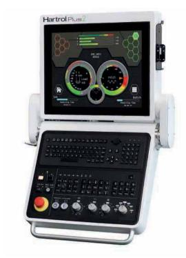
In addition to spindle load monitoring and automatic feed control, the CNC system's machine monitoring cache also incorporates a tool location display plus a work schedule management function that integrates with the Hartnet machine/operator utilisation routines.
