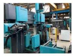
The system allows Dyfed Steels to load on new materials direct from on-site stock and remove rust and mill scale in a single pass, adding the primer paint without the need to handle the materials again until they are offloaded for the next processes.
