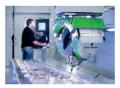
Removal of sharp edges with a milling cutter eliminates possible stress points, takes away material that could otherwise detach and cause blockage or wear, improves a component's appearance and promotes safe handling. Titanium aerospace components can be profiled so that edge radii are within ± 25 microns and surface finish is better than Ra 0.8.
