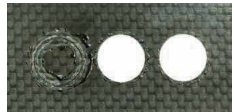
CFRP sheet cut with CO 2 laser: left hand circle Yb-doped fibre laser, middle circle and a multiple wavelength laser beam right hand circle
