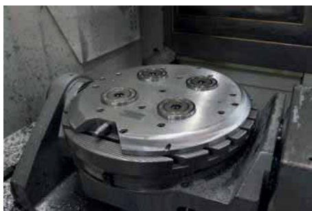
The flexibility achieved by the K20 AMF zero-point clamping system is particularly noticeable on the DMG machine
