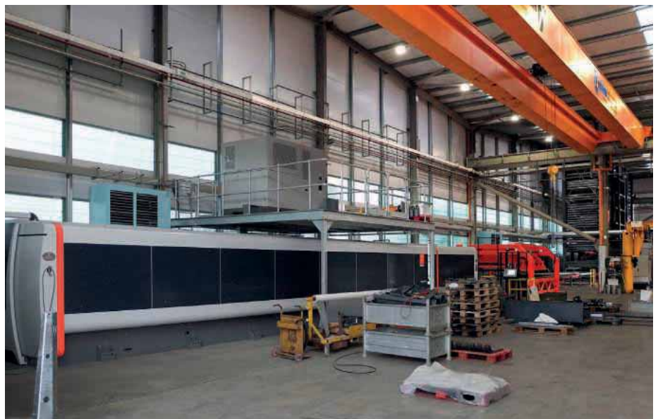
The Bystronic BySprint fibre laser cutting machine for processing 20 m stock at Inishowen Engineering. The storage towers are in the background
