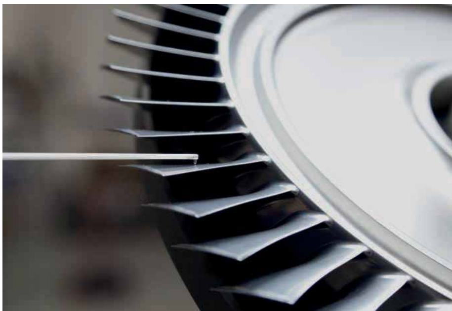
Long with smooth airflow surfaces, blisk performance greatly depends on a precise and uniform blade profile, especially along the leading and trailing edges
