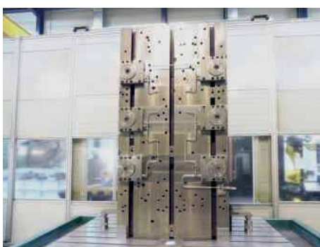
The extra-strong K40-H AMF modules are used for heavy-duty cutting
