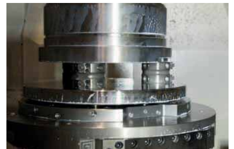
The AMF zero-point clamping modules are largely responsible for drastically shortening production times
