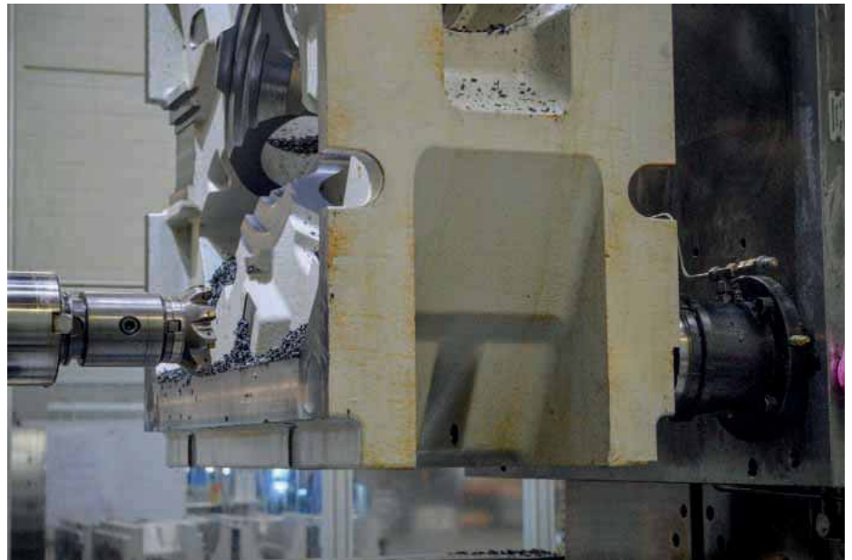
The extra-strong K40-H AMF modules with a diameter of 148 mm realise 40 kN pull-in / locking forces as well as 105 kN holding force
