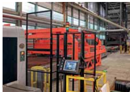
A carriage automatically conveying a 4 m x 2 m mild steel sheet from one of the storage towers to the 20 m fibre laser. Larger sheets are loaded singly onto the shuttle table
