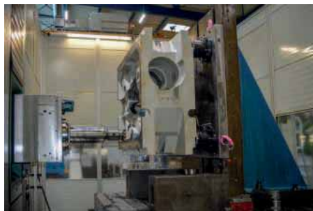
On the huge Union drilling rig for heavy-duty cutting, the extra-strong K40-H AMF modules are used for direct clamping of the workpiece
