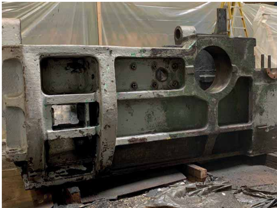
Top and below image: a 4" upsetter before and mid-progress cleaning for rebuild preparation
