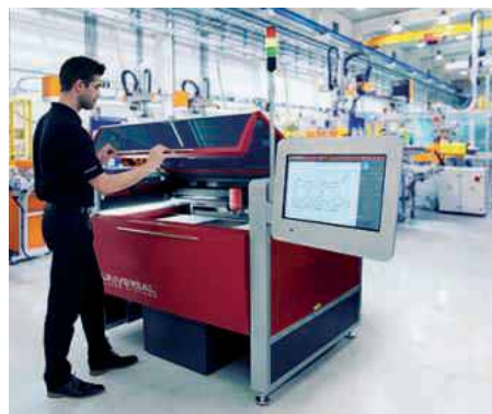
Universal Laser's ULTRA X6000 Platform uses MultiWave Hybrid Technology to combine different laser wavelengths into a single coaxial beam
