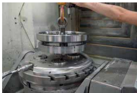
As the AMF zero-point clamping makes it so easy to re-clamp, replacement parts that are unplanned and need to be produced quickly can be incorporated into the production process without any problems
