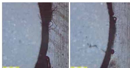
Left image: Microscopic image of the cut made using only the Yb-doped fibre laser showing significant loss of polymer matrix material and exposed carbon fibres
