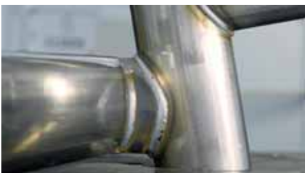
With automated welding production, gym80 achieves higher welding quality.
