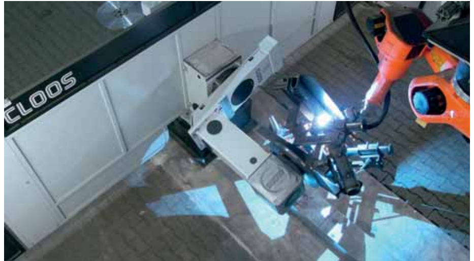
Today, gym80 uses ten CLOOS robot systems to weld a wide variety of components.
