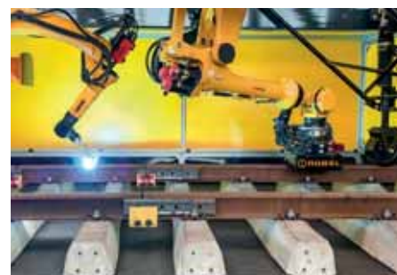
The system features a rail-traversing wagon mounted by two FANUC robots which detect internal and external defects.
