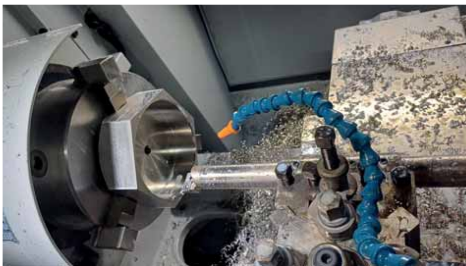
APF Services reduced the cycle time for hexagon end caps from 12 hours to 2 hours using its XYZ Proturn RLX 425.
