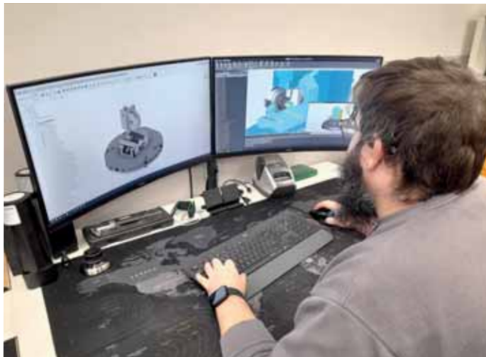
Ian Foss, CNC programmer, using Vericut to check the through-deck sheave block.
