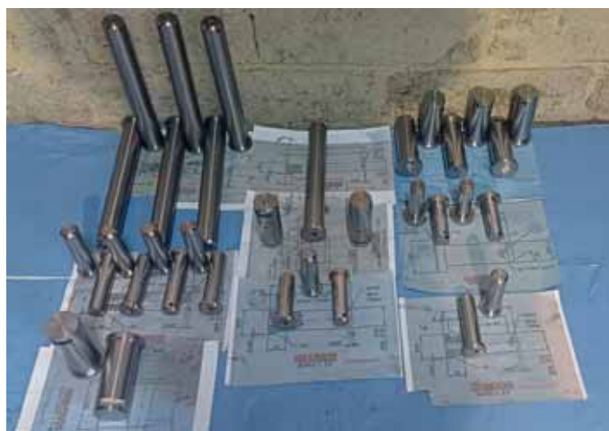
A selection of shafts turned by APF Services on its XYZ Protturn RLX 425 CNC lathe using its XYZ Protturn RLX 425.
