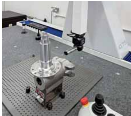
Four images of the LK Altera C 10.7.5 CMM inspecting a Spitfire axle at Rodwell Powell's Basildon facility.
