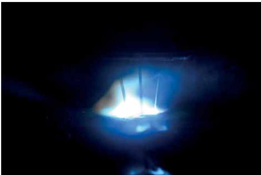
TANDEM+ combines two independent arcs with a filler wire in a molten pool.
