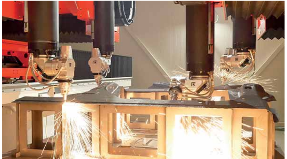
At the heart of Giga Laser Next is a unique configuration of four synchronized laser heads working simultaneously on the same part.
