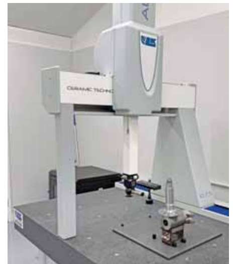
Four images of the LK Altera C 10.7.5 CMM inspecting a Spitfire axle at Rodwell Powell's Basildon facility.
