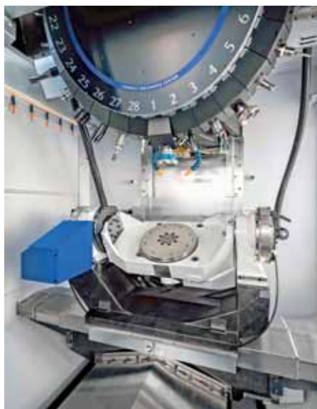
The working area of the Speedio U500Xd2-5AX 100T, which has a footprint of fractionally over 4 m 2
