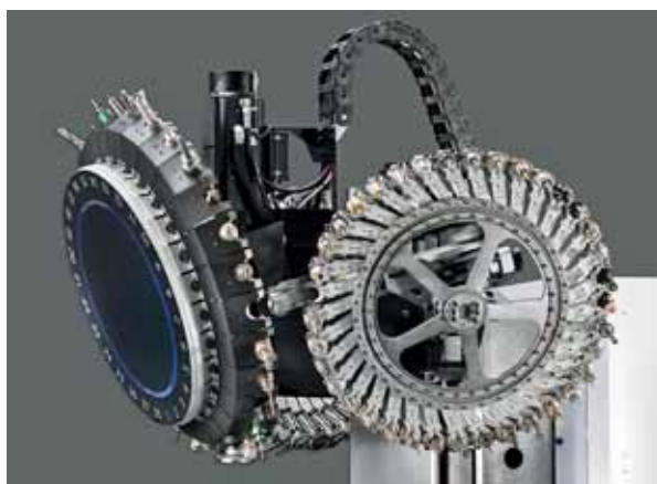
A side view of the machine, showing the mechanism for cutter exchange from a tool stocker into the turret.
